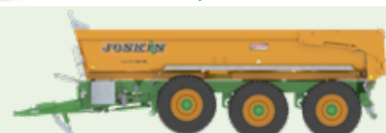
Front lifting axle (tridem) to limit wear on the road and increase the load on the tractor when needed.
